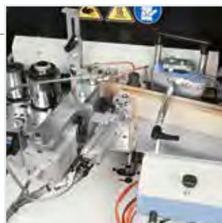
VC-V1 gluing unit: homogeneous application of the glue on all materials.
