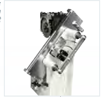
K-1 end cutting unit: double blade with independent copying devices.
