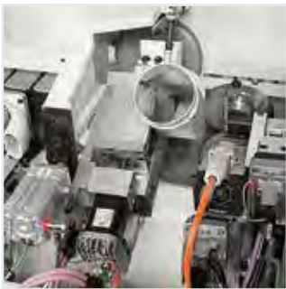
R-HP Multiedge 2R trimming unit.
