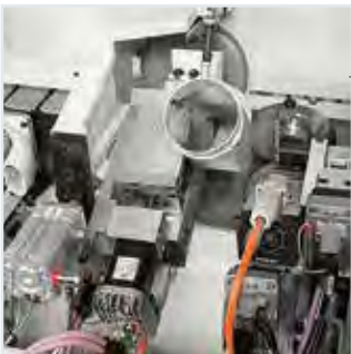
R-HP Multiedge 2R trimming unit.
