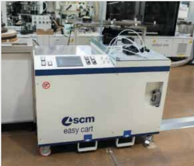
The Easy Cart device for optimising the control and maintenance of polyurethane glues was chosen by a leading manufacturer in the kitchen industry, Arclinea .
