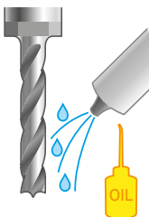
Air blower with micro-lubrication Blower with air and a small amount of oil suitable for lubricating and cooling the tool when machining non-ferrous metals.
