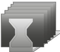
Protection of X-Y axis guides A dedicated cleaning and protection system means that even abrasive materials can be machined.
