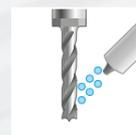
**Ionized air blower on electrospindle**
