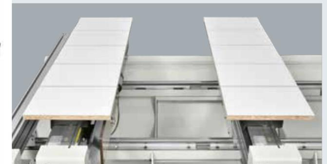
*From a single panel can be obtained more elements and automatically re-position them to carry out all machining without interrupting the production cycle; at the end the work pieces are returned to the initial position to facilitate the unloading from the work table.*
