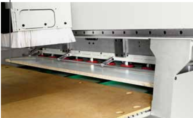
Precise and rapid panels positioning on the work table with the vacuum pods system.
