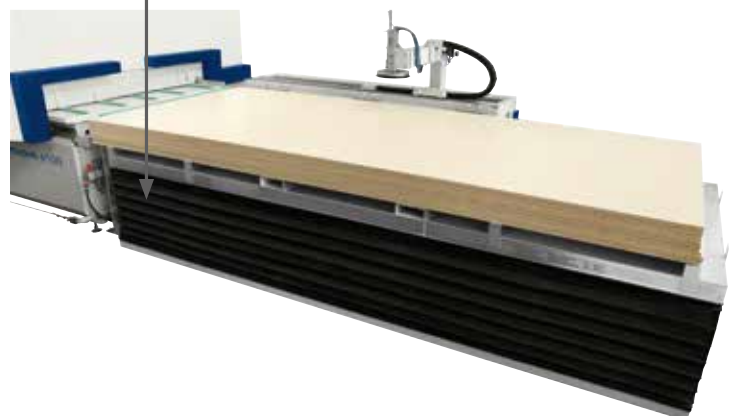
Lifting table for the management of panels stacks with height up to 700 mm.
