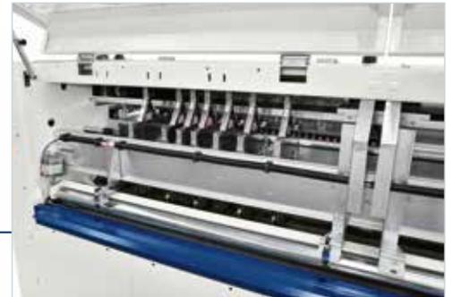
*Longitudinal cutting and creasing units*
