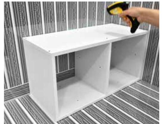
The **scanbox** allows reading the dimensions of a single or several products together and sends the data to the machine for box production. It can also be used for creating a database with the dimensions of all items.
