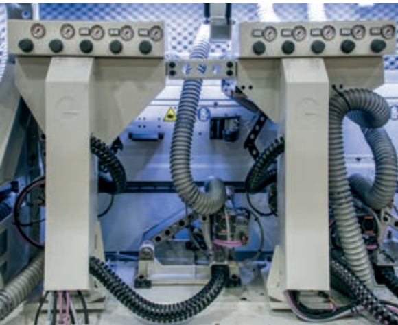
The edge is sprayed with NFly cooling solution before the panel goes through the machining section.
