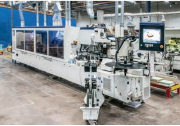
Utopia's stefani xd is equipped with a unique nesting lock system that allows pre-drilled and grooved components to be edgebanded perfectly.
