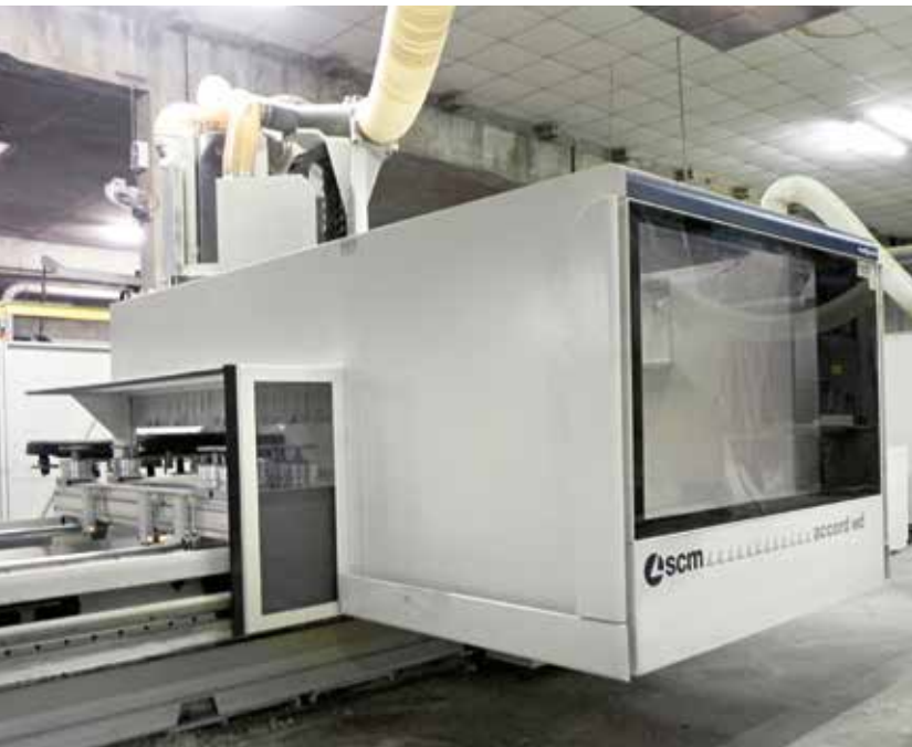
ACCORD WD WITH XILOG MAESTRO SOFTWARE ON THE MELGARI PRODUCTION LINE
