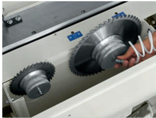
**RAPID BLADES LOCKING/UNLOCKING: MACHINING SAFETY IN A REDUCED TIME.**
